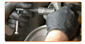
Remove the retaining springs of the brake pads.
