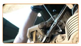
15 Remove the caliper bracket.
