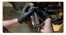
Tighten the brake caliper bracket. Use a drive socket #18. Use a torque wrench. Tighten it to 100 Nm torque.+90°
