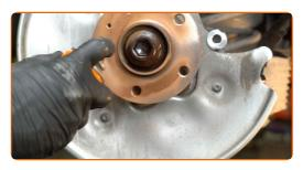
20 Install the brake disc.
