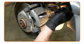
Remove the brake caliper.
