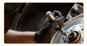
18 Remove the brake disc.
