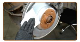
Replacement: brake discs - Audi A4 B8. Tip from AUTODOC:
