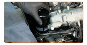
Screw the new filter into its place. Use the 76-14F socket. Use a torque wrench. Tighten it to 18 Nm torque.
