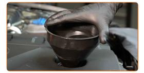
Pour oil into the engine through the filler. Required amount of oil: 4.6 L.
