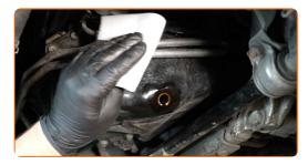
Screw in the new drainage plug and tighten it. Use Torx T45. Use a torque wrench. Tighten it to 26 nm torque.
