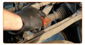
Undo the fastening nut that attaches the stabilizer link to the shock absorber fork. Use a combination spanner #16.
