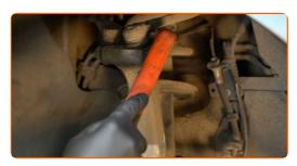
Unscrew the upper control arm fasteners (2 pieces). Use a combination spanner #16. Use a drive socket #16. Use a ratchet wrench.
