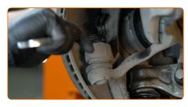
Disconnect the tie rod end from the steering knuckle.
