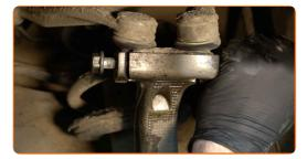
Detach the upper control arm from the steering knuckle. Use a crowbar.
