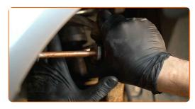
Screw in the fasteners (2 pieces) of the upper control arm. Use a combination spanner #16. Use a drive socket #16. Use a ratchet wrench.
