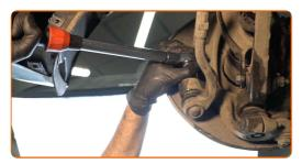
Tighten the upper control arm fasteners (2 pieces). Use a combination spanner #16. Use a drive socket #16. Use a torque wrench. Tighten it to 40 nm torque.
