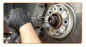
Remove the brake caliper.
