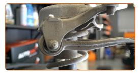
Clean the shock strut fasteners. Use a nylon cleaning brush. Use WD-40 spray.
