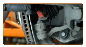
Unscrew the end fastening nut to the steering knuckle. Use a combination spanner #21.
