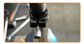
Detach the shock absorber fork from the shock strut.
