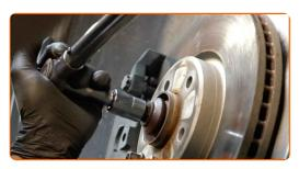
Treat the shock strut fasteners. Treat all joints of the arm. Use copper grease.
