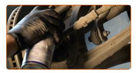
Unscrew the fasteners connecting the stabiliser link to the stabiliser bar. Use a combination spanner #16 (2 pieces).
