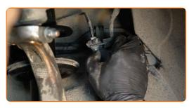
84 Attach the ABS sensor connector.
