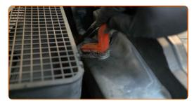
Loosen the upper fastener of the shock strut mount. Use a drive socket #16. Use a ratchet wrench.
