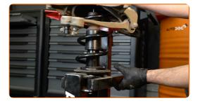
Remove the assembled shock strut.
