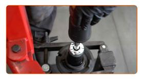
Install the spring on the shock absorber.
