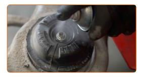
Remove the strut piston rod nut. Use a drive socket #18. Use HEX No.H6. Use a ratchet wrench.
