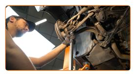
Tighten the fastener connecting the stabilizer link with the shock absorber fork. Use a combination spanner #16. Use a drive socket #16. Use a torque wrench. Tighten it to 40 Nm torque.+90°
