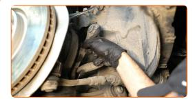
Tighten the stabiliser link fastener. Use a combination spanner #16 (2 pieces).
