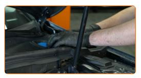
Remove the fender protection cover.
