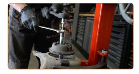
Release the coil spring.
