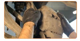
Install the brake caliper retaining spring.
