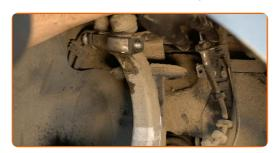
Clean the ABS sensor connector. Use a nylon cleaning brush. Use WD-40 spray.
