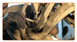
Screw in the fasteners connecting the suspension strut fork to the lower control arm. Use a combination spanner #18. Use a drive socket #18. Use a ratchet wrench.
