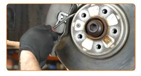
11 Remove the brake caliper.
