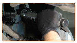
19 Install the brake caliper retaining spring.
