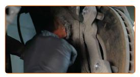
Unscrew the caliper bracket fastening. Use a drive socket #21. Use a tap wrench.
