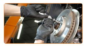
18 Remove the brake disc.
