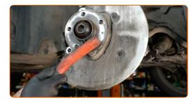
20 Install the brake disc.
