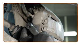
29 Install the brake caliper retaining spring.
