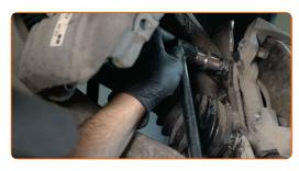
Remove the caliper bracket.
