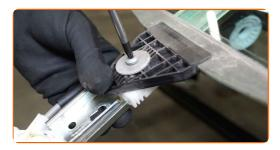
Turn the window regulator drive gear. This way you will return the glass to its standard position. Use round-nose pliers.
