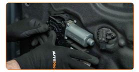
Screw in the power window motor fasteners. Use Torx T27. Use a ratchet wrench.
