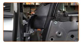
Remove the wing mirror screws. Use Torx T30. Use a ratchet wrench.
