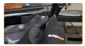
Tighten the screws of the wing mirror. Use Torx T30. Use a torque wrench. Tighten it to 15 Nm torque.
