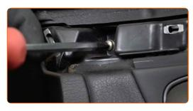
Remove the door handle screw. Use a Phillips screwdriver.
