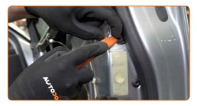
Unscrew the car door frame fasteners. Use Torx T45. Use a ratchet wrench.
