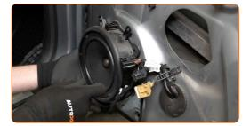
Screw in the fasteners of the speakers. Use Torx T25. Use a ratchet wrench.
