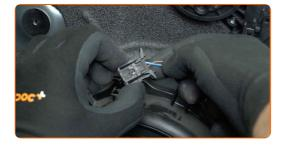
Detach the power window connectors from the control unit. Use a plastic trim tool.
