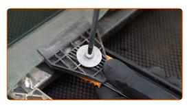
Turn the window regulator drive gear. This is how you release the glass from the window regulator drive. Use round-nose pliers.
