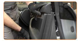
Screw in the upper fasteners of the door card. Use a Phillips screwdriver.
