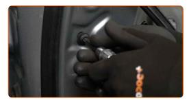
Tighten the door frame fasteners. Use Torx T45. Use a torque wrench. Tighten it to 35 Nm torque.
