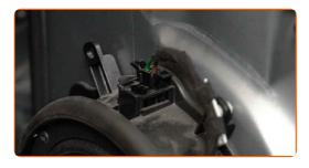
Attach the door panel sound insulation.
