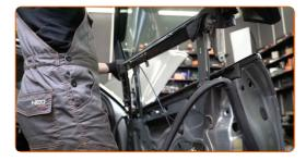
Connect the wiring of the wing mirror.
