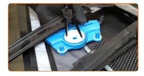
Unscrew the fasteners of the window regulator drive gear. Use Torx T25. Use a ratchet wrench.
