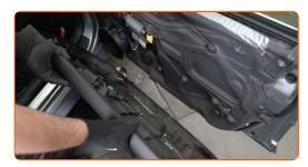
Detach the power window connector from the door panel.
