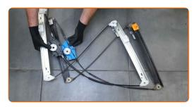
Screw in the fasteners of the window regulator drive gear. Use Torx T25. Use a ratchet wrench.
