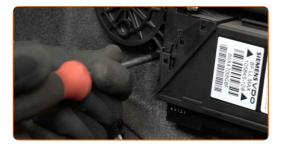
17 Remove the power window motor.
