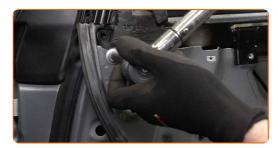
Screw in the lower fasteners of the window regulator mechanism. Use Torx T25. Use a ratchet wrench.
