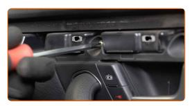
Screw in the lower fasteners of the door card. Use a Phillips screwdriver.
