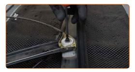
Remove the window regulator mechanism.
