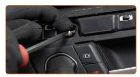
Unscrew the lower fasteners of the door card. Use a Phillips screwdriver.
