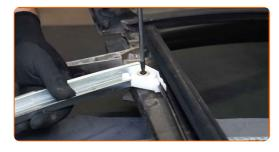
Reinstall the glass into the window regulator drive.
