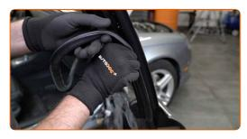
Install the door frame fastener cap.
