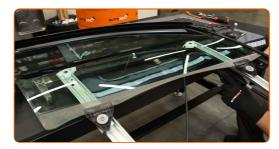
Tighten the window glass fasteners. Use Torx T20. Use a torque wrench. Tighten it to 11 Nm torque.
