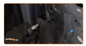
Remove the door frame fastener cap. Use a plastic trim tool.
