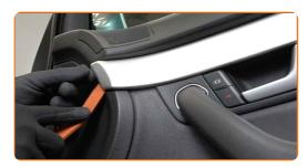
Unscrew the upper fasteners of the door card. Use a Phillips screwdriver.
