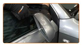
Screw in the side mirror fastener. Use Torx T30. Use a ratchet wrench.
