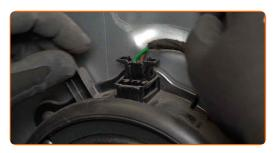
Unscrew the fasteners of the speakers. Use Torx T25. Use a ratchet wrench.
