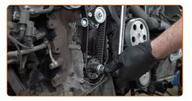
Replacement: water pump & timing belt kit – Audi A4 B7. AUTODOC recommends:
