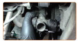
Attach the clip of the lower coolant hose.
