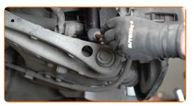
29 Screw in the lower fastener of the shock absorber. Use a combination spanner #21. Use a drive socket #21. Use a ratchet wrench.
