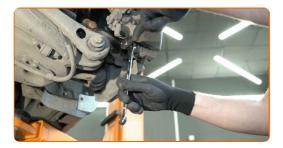
11 Remove the brake caliper.
