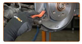
15 Install the retaining springs of the brake pads.
