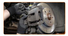
Install the parking brake cable into the brake caliper bracket. Use water pump pliers. Use pliers.
