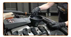
Pour oil into the engine through the filler. Required amount of oil: 4.6 l.
