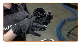
Install a new oil filter housing cover and tighten it. Use a drive socket #36. Use a torque wrench. Tighten it to 25 Nm torque.
