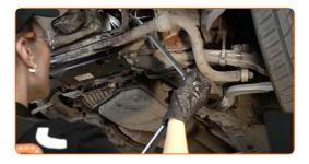
Screw on the cap of the oil filter cover.
