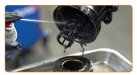
18 Install a new O-ring to its mounting seat on the filter cover.
