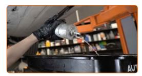
Clean the fasteners of the fuel supply lines. Use all-purpose cleaning spray.
