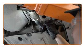
Disconnect the fuel supply lines from the fuel filter. Use a clip removal tool.
