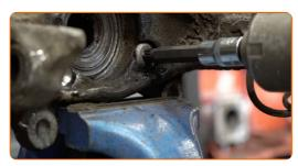
Remove the wheel hub from the steering knuckle.
