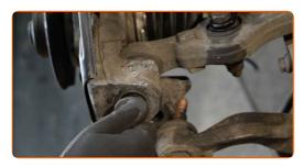
67 Connect the ball joint to the steering knuckle.
