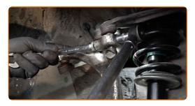
Treat all joints of the arm. Treat the fasteners of the ball joint. Treat the fastener connecting the tie rod end to the steering knuckle. Use copper grease.
