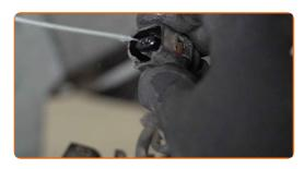
Connect the brake pad wear sensor plug.
