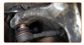
Screw on the fastening nut that connects the tie rod end to the steering knuckle. Use a drive socket #15. Use a ratchet wrench.
