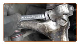
28 Remove the fastening bolt.
