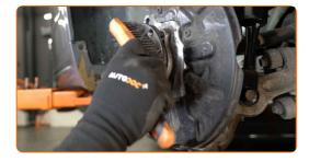
75 Install the brake disc.
