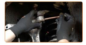
Screw in the fasteners of the upper control arms. Use a combination spanner #16 (2 pieces).
