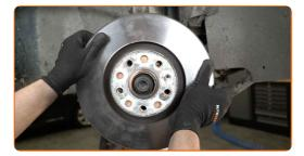
Tighten the brake disc fastening. Use Torx T30. Use a torque wrench. Tighten it to 5 Nm torque.
