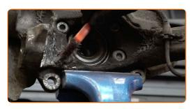
Unscrew the wheel hub axle nut. Use XZN #12. Use a ratchet wrench.
