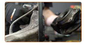
Remove the hub bearing mounting. Use a universal puller.
