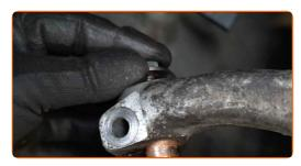
Screw in the tie rod end fastening bolt. Use a combination spanner #13.
