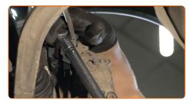
Tighten the ball joint fastener. Use a drive socket #18. Use a torque wrench. Tighten it to 110 Nm torque.
