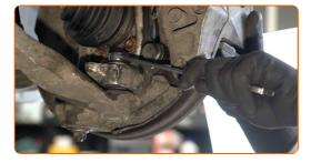
Unscrew the rear fastener connecting the control arm to the subframe. Use a combination spanner #18 (2 pieces).
