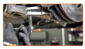
10 Remove the fastening bolt.
