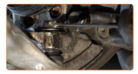
Screw the rear arm fastener. Use a combination spanner #18 (2 pieces).
