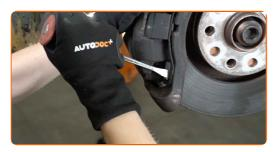
13 Remove the brake caliper.
