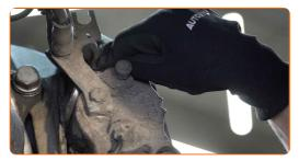
22 Install the brake caliper retaining spring. Use a crowbar.
