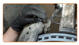
Connect the brake pad wear sensor plug.
