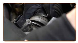
18 Fasten the clamp on the air intake hose. Use clic-R collar pliers.
