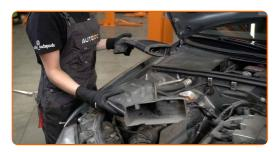
Unplug the mass air flow sensor connector.
