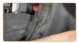
Remove the fender protection cover.
