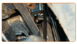
Place the serpentine belt on the crankshaft pulley.
