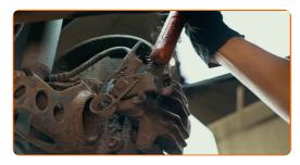
Unscrew the brake caliper fastening. Use a combination spanner #13. Use a combination spanner #15. Use a ratchet wrench.
