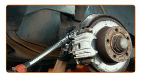
Install the parking brake cable into the brake caliper bracket. Use water pump pliers. Use a crowbar.
