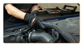
Unscrew the fasteners of the cowl grille. Use Torx T20. Use a flat screwdriver.
