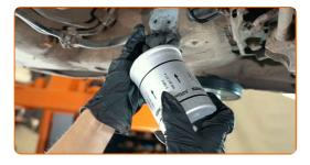
13 Install the fuel filter bracket.
