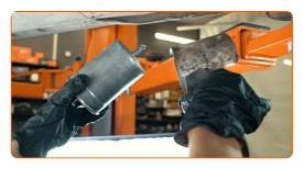
12 Attach the pipe to the fuel filter.
