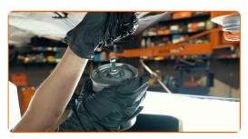
Remove the fuel filter bracket.
