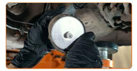
Attach the pipe to the fuel filter.
