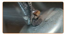
Loosen the fastening clamps of the fuel filter pipes. Use a flat screwdriver.
