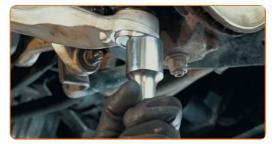
Screw the fastener connecting the control arm to the subframe. Use a combination spanner #18.
