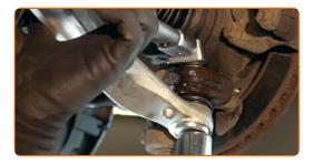
Remove the support from under the arm.
