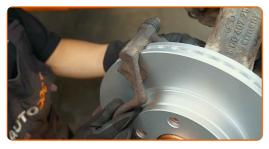
Tighten the brake caliper bracket. Use a drive socket #17. Use a torque wrench. Tighten it to 125 Nm torque.
