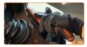
Unscrew the caliper bracket fastening. Use a drive socket #17. Use a ratchet wrench. Use a tap wrench.
