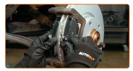
Install the brake caliper and fix it. Use a combination spanner #15. Use a drive socket #13. Use a torque wrench. Tighten it to 30 Nm torque.
