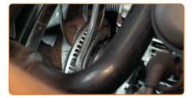
Loosen the alternator fasteners. Use HEX No.H8.
