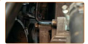
Unscrew the fastener of the viscous fan clutch. Use a combination spanner #46. Use HEX No.H8.
