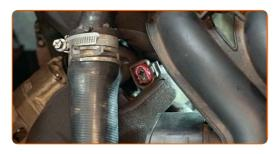
Unscrew the alternator power cable fastener. Use a combination spanner #13.
