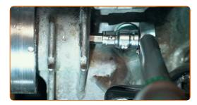
Pull aside the V-ribbed belt tensioner pulley. Use a combination spanner #17.
