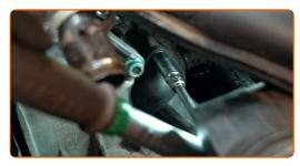
Tighten the alternator power cable fastener. Use a drive socket #13. Use a torque wrench. Tighten it to 5 nm torque.
