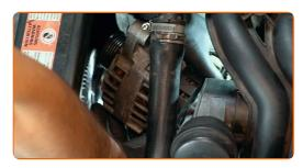
Disconnect the alternator connector.
