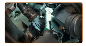
Connect the alternator connector.
