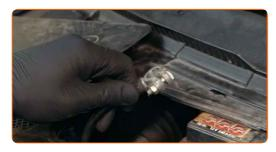
Loosen the alternator fasteners. Use HEX No.H8.
