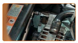
Tighten the fastener of the viscous fan clutch. Use a combination spanner #46. Use HEX No.H8. Use a torque wrench. Tighten it to 24 nm torque.
