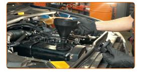
Pour oil into the engine through the filler. Required amount of oil: 3.5 l.
