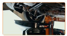
Clean the area of the oil pan drainage hole. Clean the oil filter. Use a wire brush. Use all-purpose cleaning spray.
