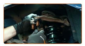
Detach the driveshaft from the steering knuckle.
