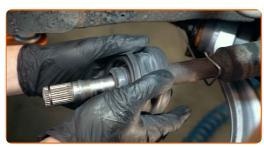
37 Install the CV joint circlip.
