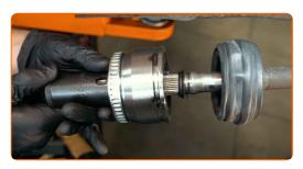
Move the inner race of the CV joint from side to side to bed it in.
