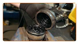
Remove the CV joint bearing. Use a crowbar.
