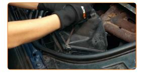
Slightly raise the cover of the air filter housing.
