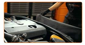
Detach the air duct housing from the air filter housing.
