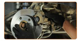
Use a combination spanner #13. Use a combination spanner #15. Use a torque wrench. Tighten it to 35 Nm torque.
