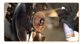
17 Install the brake disc.
