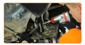
Tighten the fastener connecting the stabilizer link to the stabilizer bar. Use a combination spanner #17. Use HEX No.H5. Use a torque wrench. Tighten it to 60 Nm torque.
