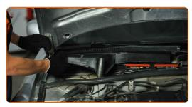
Install the cowl grille clips. Use a flat screwdriver.
