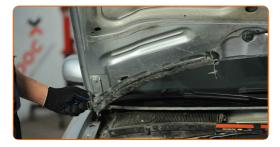
Remove the cabin filter. Use a flat screwdriver.
