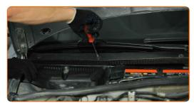
Screw in the fasteners of wiper cowl grille located on the right side. Use a drive socket #8. Use a ratchet wrench.
