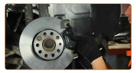
27.1 Install the brake caliper and fix it.
