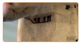
11 Remove the brake caliper.
