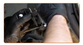
Loosen the lock nut securing the tie rod end to the tie rod. Use a combination spanner #23. Use a combination spanner #24.
