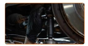
Tighten the tie rod end locknut. Use a combination spanner #24 (2 pieces). Use a torque wrench. Tighten it to 50 nm torque.
