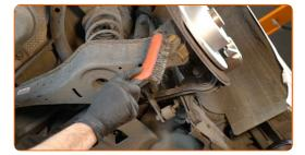
Make a mark on the camber adjustment bolt.
