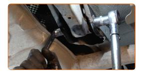
Tighten the fastener connecting the suspension arm to the rear knuckle. Use a combination spanner #18. Use a drive socket #18. Use a torque wrench. Tighten it to 90 Nm torque.+90°
