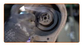
Install the coil spring together with the rubber mounts into the mounting seats.
