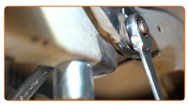
Remove the support from under the arm.
