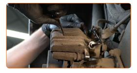
Remove the brake caliper. Use a crowbar.
