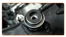
Screw the new filter into its place. Use the 76-14F socket. Use a torque wrench. Tighten it to 25 Nm torque.
