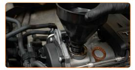
Pour oil into the engine through the filler. Required amount of oil: 3.8 l.
