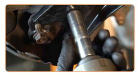
Install the rear fastener of the arm.
