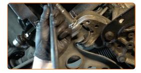
Unscrew the rear fastener connecting the control arm to the car body. Use a drive socket #18. Use a tap wrench.
