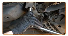
Unscrew the rear fastener connecting the control arm to the subframe. Use a drive socket #16. Use a tap wrench.
