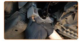
Screw the rear fastener connecting the control arm to the car body. Use a combination spanner #18. Use a drive socket #18. Use a ratchet wrench.
