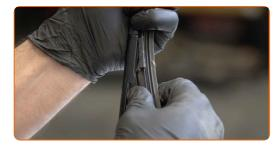
Remove the blade from the wiper arm.
