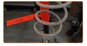
Install the spring on the shock absorber.
