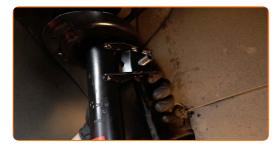
Tighten the stabiliser link fastener. Use a drive socket #18. Use a ratchet wrench.
