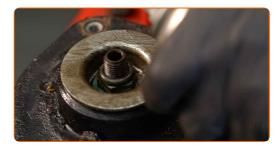
Remove the strut piston rod nut. Use HEX No.H7. Use a drive socket #21. Use a ratchet wrench.
