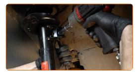
Tighten the lower fasteners connecting the shock strut to the steering knuckle. Use a drive socket #18. Use a torque wrench. Tighten it to 70 Nm torque.+90°
