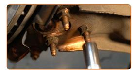
Install and tighten the drive shaft bolt. Use a drive socket #24. Use a ratchet wrench.
