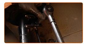
Tighten the ball joint fastener. Use a drive socket #16. Use a torque wrench. Tighten it to 60 nm torque.
