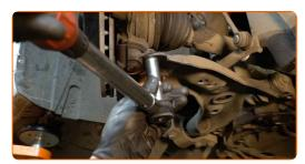
Treat the shock strut fasteners. Treat all joints of the arm. Use copper grease.
