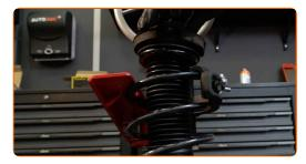
Tighten the shock strut piston rod nut. Use HEX No.H6. Use a drive socket #21. Use a torque wrench. Tighten it to 60 Nm torque.
