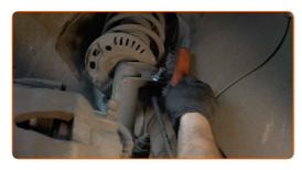
Unscrew the fastener connecting the stabilizer link to the shock strut. Use a drive socket #18. Use a ratchet wrench.
