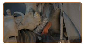
Unscrew the lower fastener connecting the shock strut to the steering knuckle. Use XZN #14. Use a drive socket #18. Use a tap wrench. Use a ratchet wrench.
