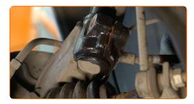
Unscrew the fastener connecting the drive shaft to the wheel hub. Use a drive socket #24. Use a ratchet wrench.
