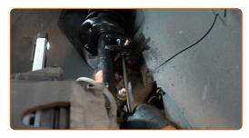
Tighten the stabiliser link fastener. Use a combination spanner #18. Use a drive socket #18. Use a ratchet wrench.
