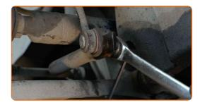
Unscrew the fastener connecting the stabilizer link to the shock strut. Use a drive socket #18. Use a ratchet wrench.
