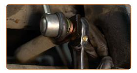
Tighten the fastener connecting the stabilizer link to the shock strut. Use a drive socket #18. Use a torque wrench. Tighten it to 65 Nm torque.
