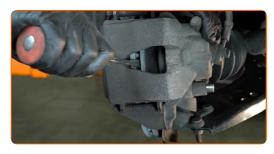
10 Remove the brake caliper.
