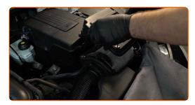
Unscrew the air filter housing bracket. Use a Phillips screwdriver.
