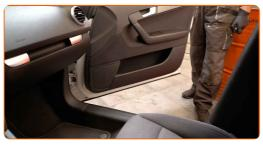
Unscrew the fasteners of the bottom trim panel.
