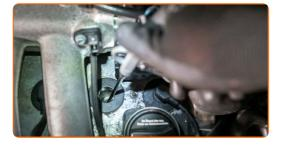
Unscrew the spark plugs. Use the spark plug socket #16.
