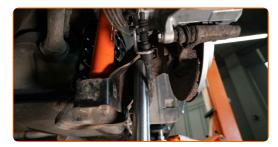
Tighten the lower fastener of the shock absorber. Important! Be sure to use new fasteners. Use a combination spanner #16. Use a drive socket #16. Use a torque wrench. Tighten it to 40 Nm torque.+90°
