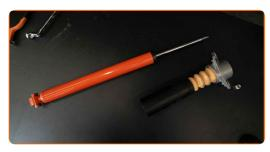
Install the top mount on the new shock absorber and secure it. Use a combination spanner #16. Use an adjustable wrench. Use a torque wrench. Tighten it to 25 Nm torque.
