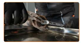
Remove the shock absorber mount, boot and bump stop.
