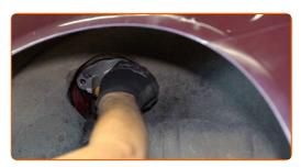
Tighten the top shock absorber fastening. Important! Be sure to use new fasteners. Use a drive socket #16. Use a torque wrench. Tighten it to 30 Nm torque.+90°
