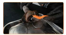
Remove the shock absorber piston rod fastening. Use a combination spanner #16. Use an adjustable wrench.
