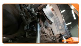
Unscrew the lower fastener of the shock absorber. Use a combination spanner #16. Use a drive socket #16.
