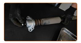
Tighten the shock absorber mount fasteners. Use a combination spanner #16. Use an adjustable wrench. Use a torque wrench. Tighten it to 25 Nm torque.
