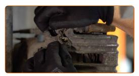
Detach the parking brake return spring. Use water pump pliers.
