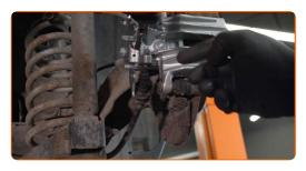
Install the return spring of the parking brake mechanism.
