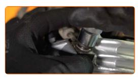
Remove the brake hose clamp.
