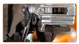
Attach the parking brake cable to the parking brake mechanism.
