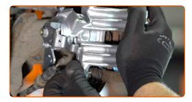
Install the parking brake cable into the brake caliper bracket. Secure the parking brake cable with the retaining clip.
