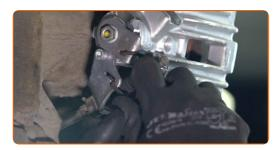
Unscrew the plug from the brake hose mounting seat on the brake caliper. Use a ratchet wrench. Use HEX No.H6.
