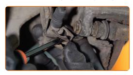
Disconnect the parking brake cable from the caliper. Use water pump pliers.
