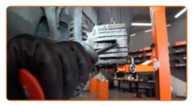
Clean the area where the brake hose is connected to the caliper, and the guide pins area. Clean the brake caliper fasteners. Use a wire brush. Use a brake cleaner.
