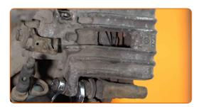
19 Remove the brake caliper.
