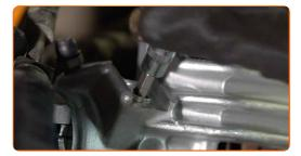
Install the brake hose to the new brake caliper.
