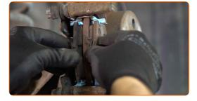
Install the brake caliper and fix it.
