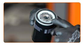
Screw the new filter into its place. Tighten it to 20 nm torque. Use a torque wrench. Use the 65/67-14f socket.
