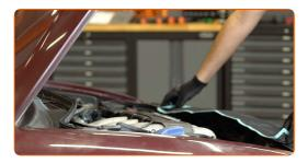
Remove the fender protection cover.
