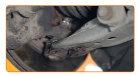
Screw in the fasteners of the ball joint lock plate (3 pieces). Important! Be sure to use new fasteners. Use a drive socket #13. Use a torque wrench. Tighten it to 20 Nm torque.+90°
