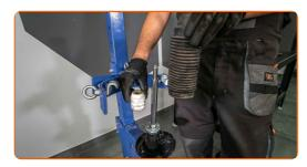
Remove the old shock absorber from the hydraulic coil spring compressor.
