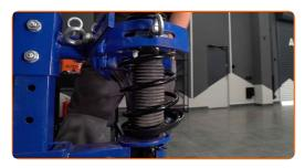
Remove the assembled shock strut.
