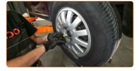
Tighten the drive shaft nut. Use 1-3/16" drive 12-point socket. Use a torque wrench. Tighten it to 180 Nm torque.
