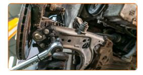
Screw the nut of the drive shaft.
