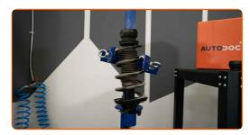
Remove the strut piston rod nut. Use flare nut socket #22. Use HEX No.H6.
