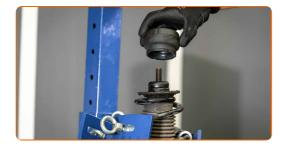
Release the coil spring.
