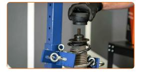
Tighten the shock strut piston rod nut. Use a combination spanner #19. Use HEX No.H6. Use a torque wrench. Tighten it to 60 Nm torque.
