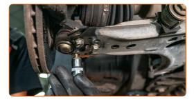
Disconnect the spherical joint from the arm.
