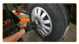
Tighten the drive shaft nut. Use 1-3/16" drive 12-point socket. Use a torque wrench. Tighten it to 180 Nm torque.
