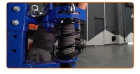
Remove the assembled shock strut.
