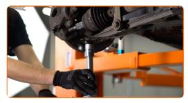
Unscrew the lower fastener connecting the shock strut to the steering knuckle. Use a combination spanner #18. Use a drive socket #18.
