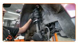
Tighten the upper fastening nut of the shock absorber strut. Do not tighten it.
