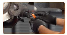
Treat the shock strut mounting seat on the steering knuckle. Use WD-40 spray.
